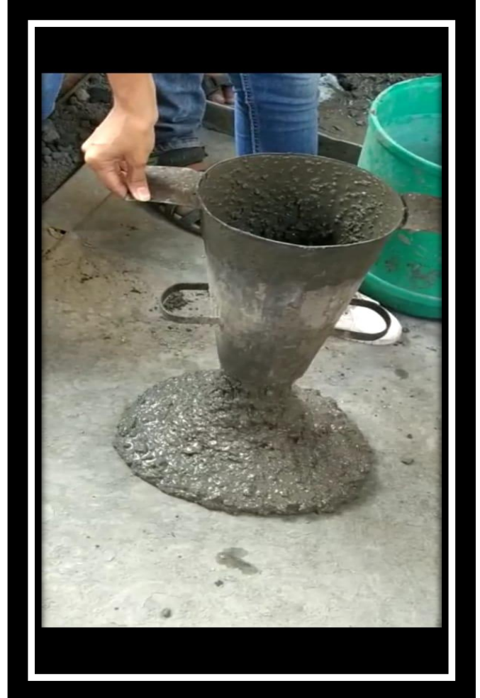
Flow test on SCC
